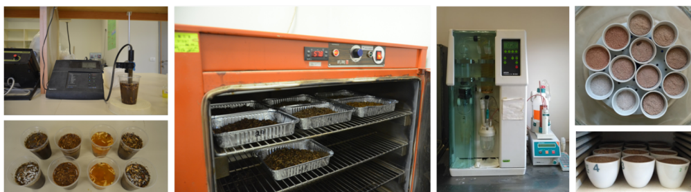
Figure 2: Chemical parameters tests (from left to right); pH and electric conductivity, water, nitrogen and ash contents.
